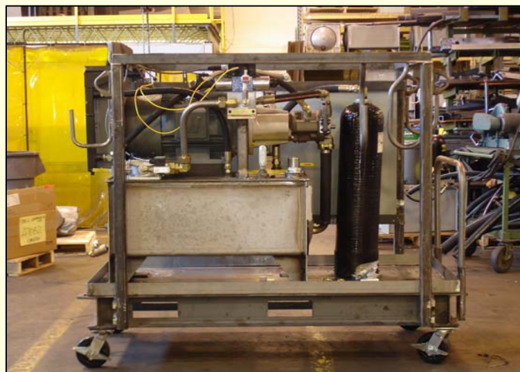
hydraulic pump unit
