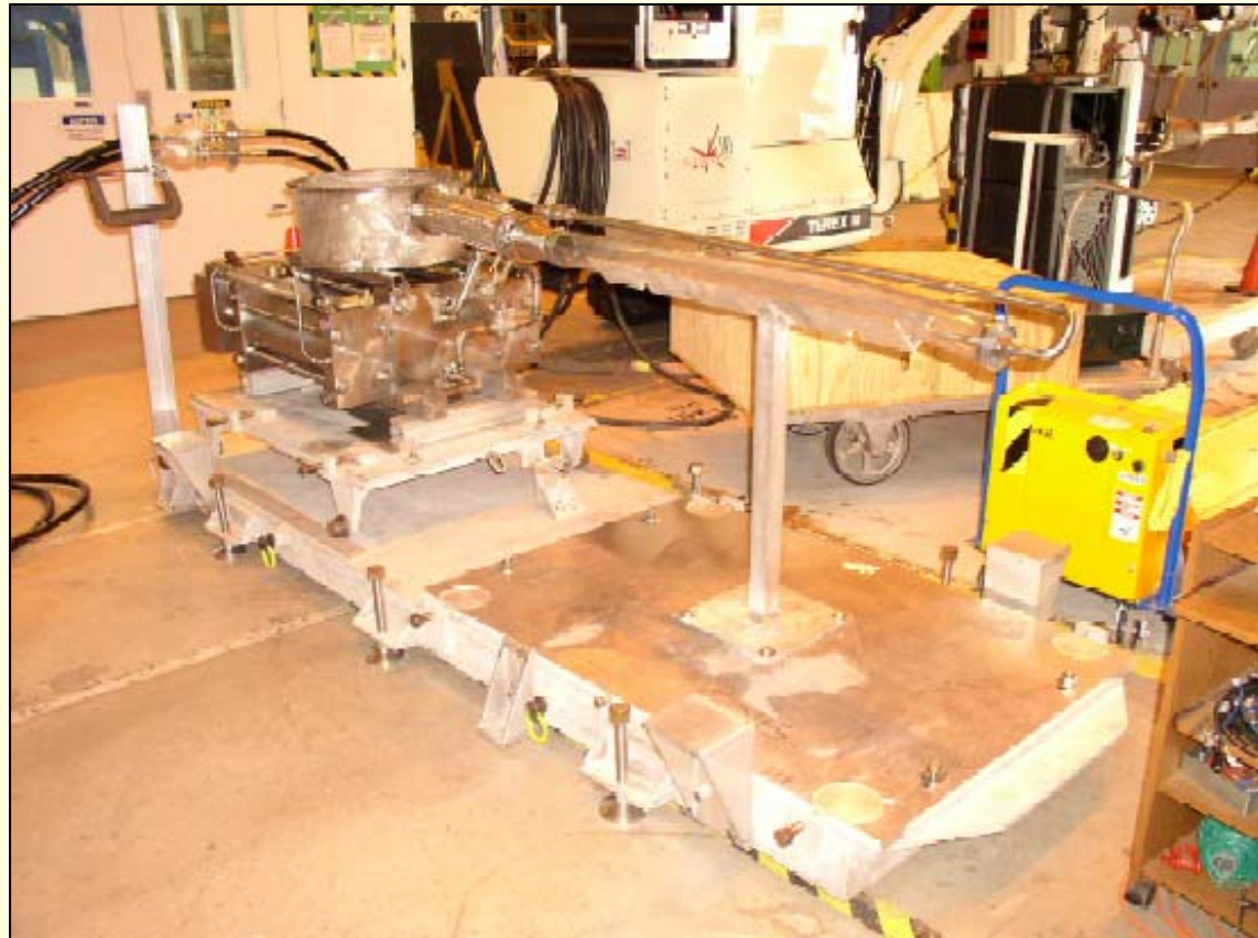
Hg-loop assembled - during water tests @ORNL
