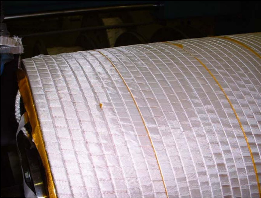
Photo taken by Dave Rakos at Everson 09-08-04. Kapton layer spaced at every eighth turn relieves axial tension in the layers near the cooling channels.
