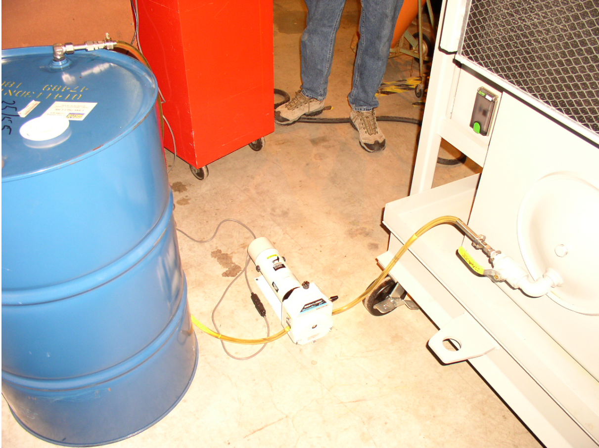
Figure X.1: Hydraulic Fluid Drain
