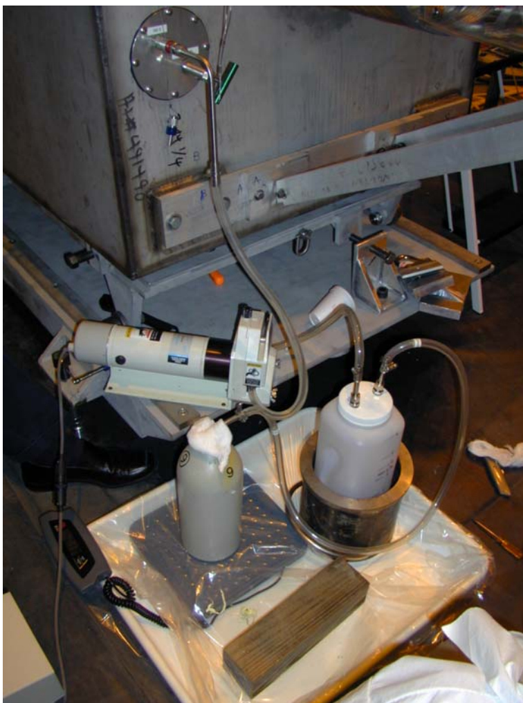
Figure VIII-2. Hg drain setup
