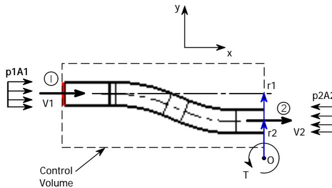
$$\rho := 13540 \frac{\text{kg}}{\text{m}^3} \quad \text{Fluid density} \quad Q := 1.57 \frac{\text{liter}}{\text{s}} \quad \text{Flow rate}$$
