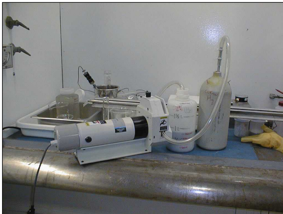
Figure 36. Peristaltic pump for transferring mercury.
