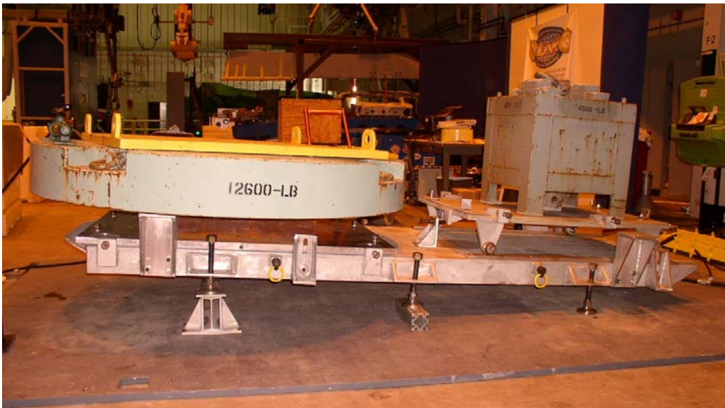
Figure 32. Baseplate load testing
