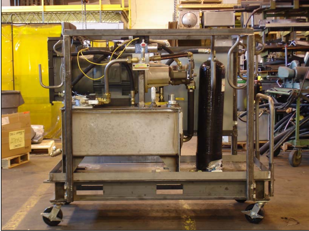
Figure 16. Hydraulic pump system.
