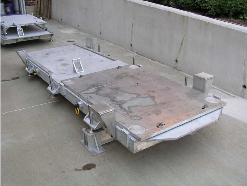
Figure 25. Common baseplate and support beam.
