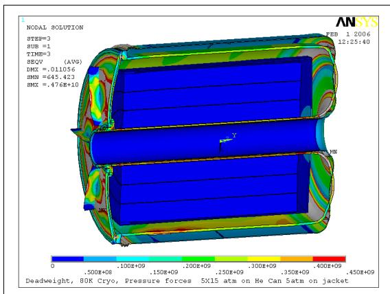
Large Displacement Analysis with 5 time the Design Pressures was Bounded.
