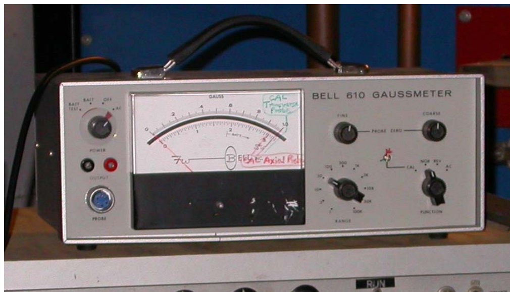
After a day warm up. It zeroed properly and read 60 milliT
