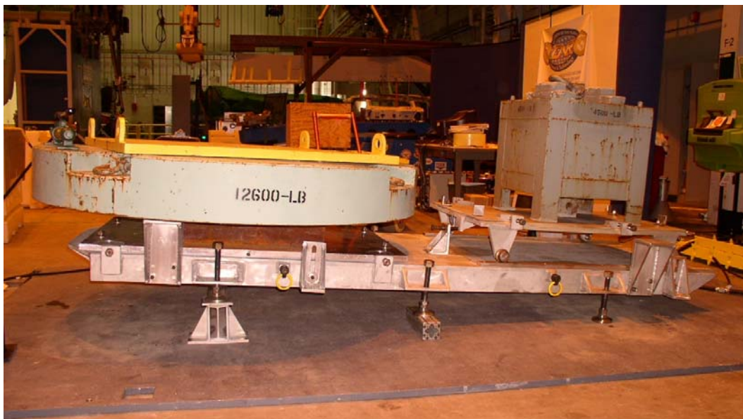
Figure 32. Baseplate load testing
