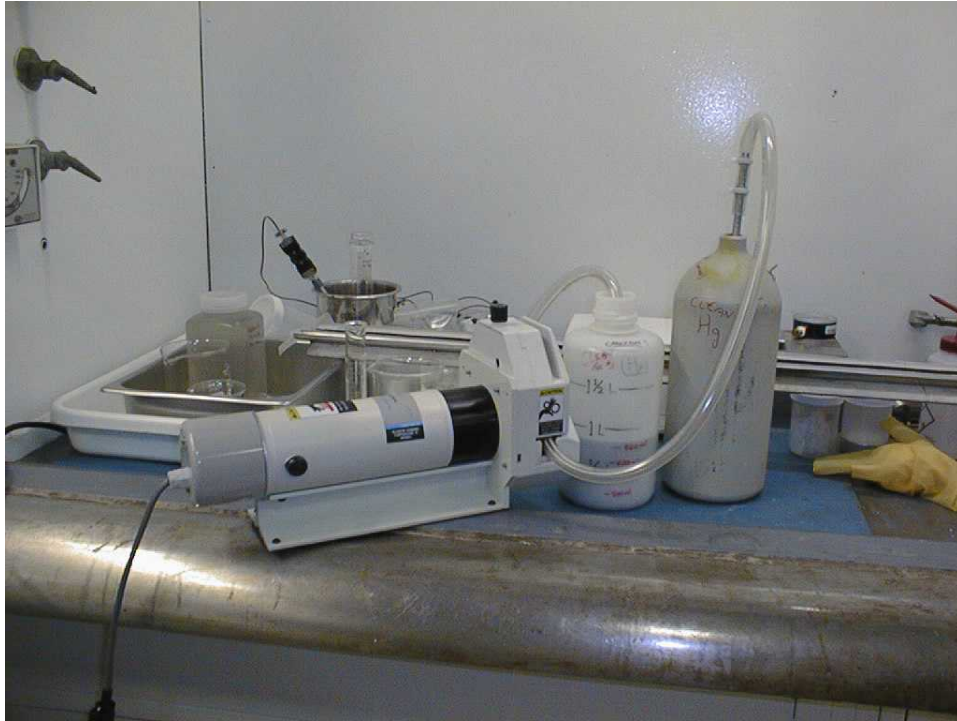
Figure H-1. Tube pump test setup; M & C Division fume hood.
