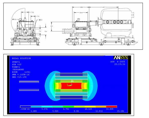
This sounds like a large force, but I am not surprised after experimenting with a small wrench in the bore of one of the coil segments at Everson. It was being heated by running it with 250 amps DC, and the force was enough to take the wrench out of your hand if you weren't careful. At 15 T there are 3 segments with 7200 amps in them. Load calculations require a non-linear
